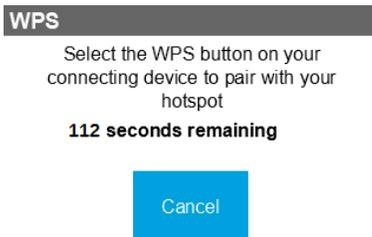
6. Within two minutes, press the **WPS key** on the wireless device you want to connect.
