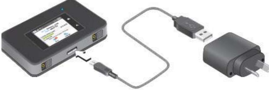
2. Plug the wall charger into a wall socket.
