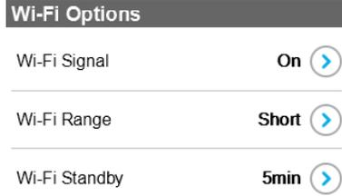
5. To disable the Wi-Fi signal in a restricted area, tap the > button next to Wi-Fi Signal.
