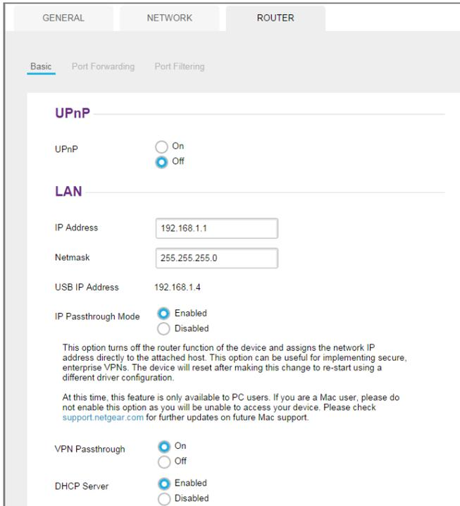
5. In the LAN section, select the On radio button next to VPN Passthrough.
