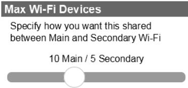
6. Slide the button to specify how you want the Wi-Fi devices to be shared between each Wi-Fi network.
