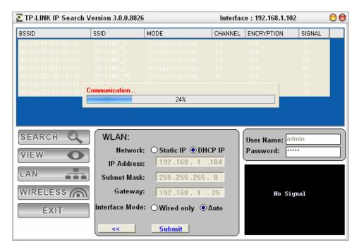
Once this step is finished, IP Search will prompt you to unplug the Ethernet cable to activate wireless access. Then IP Search will prompt you to test wireless setting or finish wireless procedure as below.
