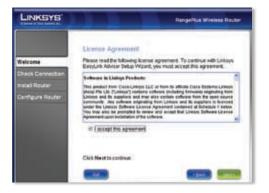
F. The Linksys EasyLink Advisor (LELA) Setup Wizard displays a series of screens that will guide you through the Router's physical installation and setup. Follow the instructions in these screens.
