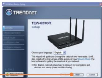
Note: Leave the **“No, thanks...”** box unchecked in order to install Network Magic immediately after the router setup.
