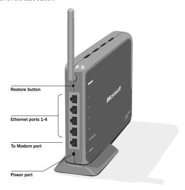
On the back of the base station, you will find a Power port, a To Modem port, four numbered Ethernet ports, and a Restore button.
