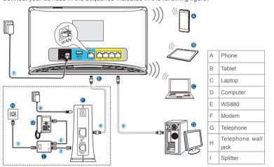
When configuring the WS880 for the first time, use a network cable to connect the WS880 to a computer.
