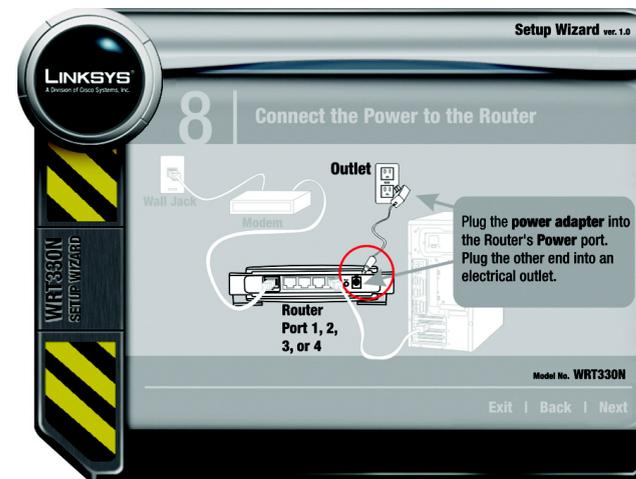
**IMPORTANT:** Make sure you use the power adapter that is supplied with the Router. Use of a different power adapter could damage the Router.
