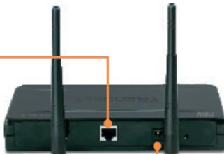
3. Connect the AC Power Adapter to the Access Point and then to a power outlet.
