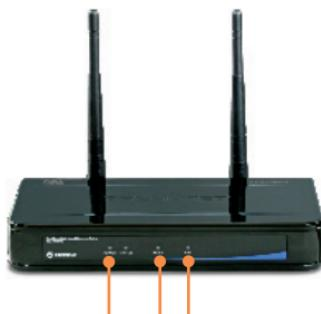
4. Verify that the following panel lights are on: **Power**, **WLAN** and **LAN**.
