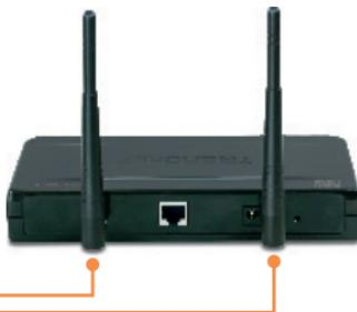
2. Connect a RJ-45 cable from the Switch/Router to the **LAN** port on the Access Point.
