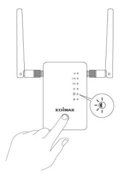
**3.** The devices will establish a connection. The extender's green WPS LED should display on for 30 seconds to indicate a successful connection.
