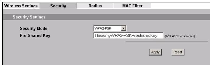
The screenshot shows the 'Security' tab in the 'Wireless Settings' window. Under 'Security Settings', the 'Security Mode' is set to 'WPA2-PSK'. The 'Pre-Shared Key' field contains the text 'ThisismyWPA2-PSKPresharedkey' and is limited to 8-63 ASCII characters. There are 'Apply' and 'Reset' buttons at the bottom right.
