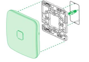
the access point. Attach the universal mounting plate with the smooth side against the wall to a junction box using the designated screw holes. Connect the small Ethernet cable (included) to the female connection in the wall, then pull it through the mounting plate and plug into Ethernet 1. Connect any passthrough device to Ethernet 2 and position the cable in the bottom channel of the access point. Next, place the access point over the mounting plate and slide down until it locks
