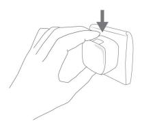
3. The devices will establish a connection. The extender's LED should display on (green) for 30 seconds to indicate a successful connection.
