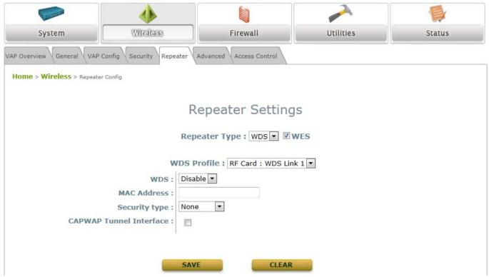
To extend the wireless coverage, EAP747 supports up to 4 WDS links for connecting wirelessly to other WDS-capable APs (peer APs). By default, all WDS profiles are disabled.
