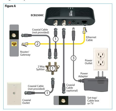
Plug one end of the Yellow Ethernet Cable into an Ethernet Port on your Router/Gateway. Plug the other end into the Ethernet Port on the back of the ECB2500C.
