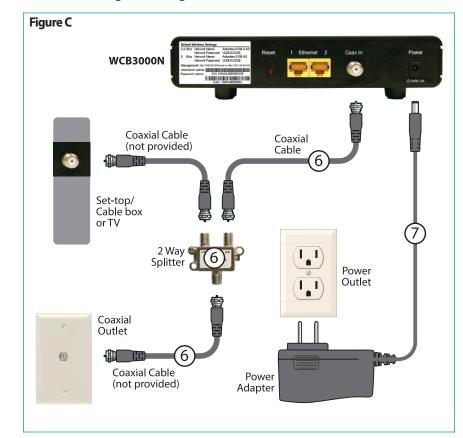
Step Connect the Coaxial Cable to the Coaxial Outlet as shown in either Figure C or D. Make sure you are using the appropriate diagram for your home as described in Step 5.
