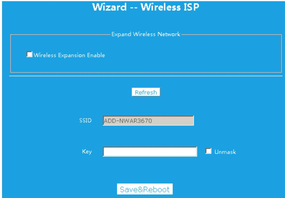
3. The SSID of the target network will be automatically filled into SSID box. Then enter the network key of the target network.
