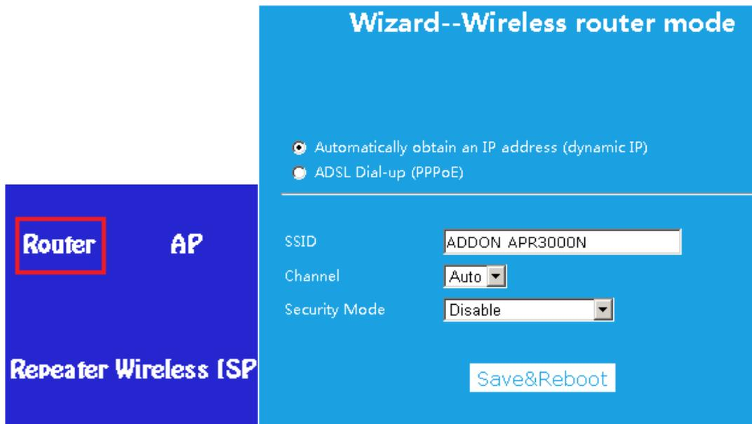
2. If you use WiFi Range Extender as a router, you don't need to configure the device and will get Internet instantly. All you need to do is to connect the ADSL or Cable Modem to the WAN port on the WiFi Range Extender (refer to figure 1).
