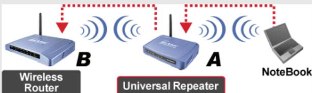
Universal Repeater doesn't require the remote device to have WDS function
