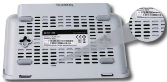
To reset the Air 4240 to the default factory settings, While the device is on, press and hold the reset button at the bottom of the device with the tip of a pencil or similar pointed object for 5 seconds
