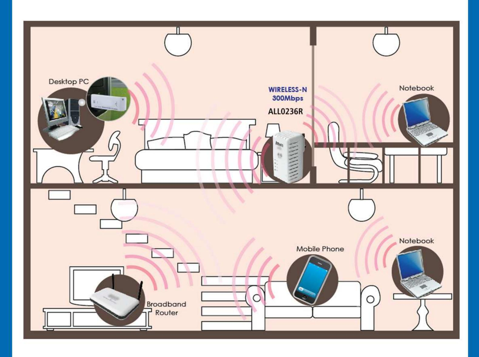
NOTE: Placement of the Wireless Repeater is crucial to get the best possible results for extending your existing wireless signal. It is ideal for the wireless repeater to be placed in a location where it can receive good wireless signal from the wireless router/AP so as to avoid disconnection and packet loss.
