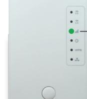
The Range Extender is equipped with a Signal Strength LED on the front of the device to help you find the most optimal location. After setup, the LED can be your guide for positioning the Extender to a better location (if needed). It may take 1-3 minutes for the LED to register after powering on the Extender. For optimal performance, we recommend a signal strength of at least 70%.
