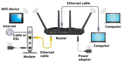
You can use a wired connection to connect a computer to the router, or you can use a WiFi connection to connect a computer or WiFi device to the router:
