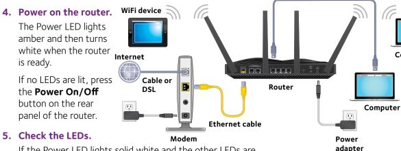
If the Power LED lights solid white and the other LEDs are off, press the **LED** button on the front panel of the router.
