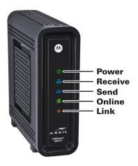
During normal operation, the POWER, RECEIVE, SEND, and **ONLINE** LEDs should always be lit SOLID. The LINK LED should FLASH during data transfer.
