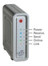
During normal operation, the POWER, RECEIVE, SEND, and ONLINE LEDs should always be **ON**. The LINK LED should **FLASH** during data transfer.
