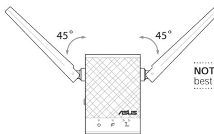
NOTE: Orient the two antennas at 45° angle for the best performance.
