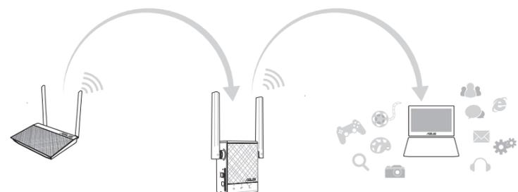
Your RP-AC51's wireless network name (SSID) changes to your existing Wi-Fi network name, ending with **\_RPT** or **\_RPT5G** and shares your router/AP's Wireless Password.
