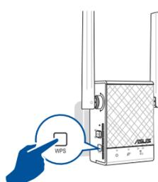
**NOTE:** Wait until the existing network LED blinks for about two (2) minutes, then turns solid blue, indicating the WPS process is completed.
