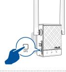
NOTE: Wait until the existing network LED blinks for about two (2) minutes, then turns solid blue, indicating the WPS process is completed.
