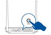
2. Press the WPS button on your RP-AC66 for more than two (2) seconds until the LEDs start to blink.
