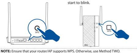
The power LED flashs for about two (2) minutes and then turns solid green. The color of the LED indicates the Wi-Fi signal strength.
