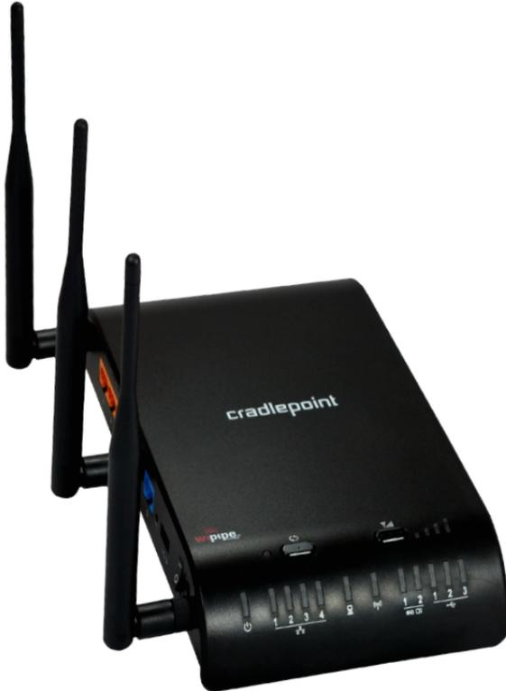
The CradlePoint Mission-Critical Broadband Router (MBR1400) is built to provide an instant network connection with high-speed 4G LTE.
