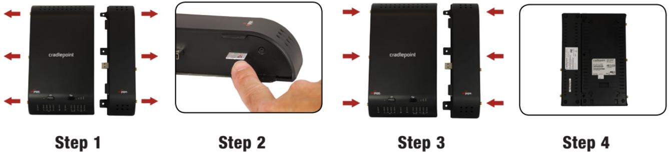
1. Disconnect the modem from the router by pulling from side to side. If you experience difficulty, apply slight pressure to the back of the device to facilitate separation.
