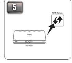
For WPS Setup, press and hold the WPS button on the DAP-1533 for about 1 second. The WPS LED will blink.
