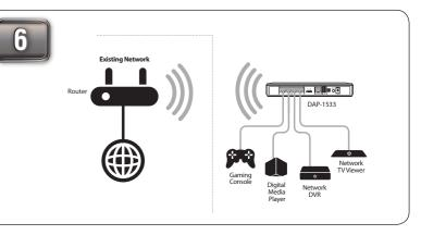
Once finished, you may connect up to 4 Ethernet (wired) devices to the DAP-1533 and connect to your existing wireless network. Note that wireless devices cannot connect to the DAP-1533 wirelessly when in MediaBridge mode.
