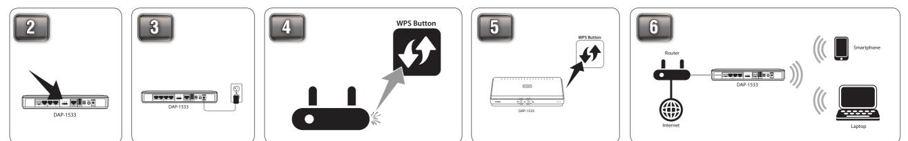
With the DAP-1533 powered off, slide the selector on the back of the device to AP 2.4GHz or AP 5GHz.
