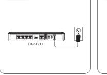
With the DAP-1533 powered off, slide the selector on the back of the device to **BRIDGE**. Attach the power adapter to a power outlet or surge protector. If the Power LED is not lit, press the Power button to turn on.
