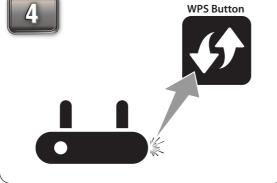
Press the WPS button on your existing wireless router or access point. The WPS LED will start to blink.
