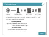
Setup is now complete. Allow about two minutes for the DAP-1860 reboot. Verify that the Status light is green and the signal strength indicators are lit. You can now unplug the DAP-1860 and connect to a different location if needed.
