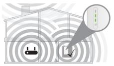
For best performance, place your DAP-1860 in between your router and your dead zone, making sure it's placed in a location where the Wi-Fi signal is still strong. Use the Smart Signal Indicator to help find a location with a strong signal. The more bars lit on the signal indicator, the stronger the Wi-Fi signal is.
