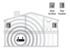
A Range Extender only works as well as the signal it is extending. Therefore, proper placement of your DAP-1860 is important in achieving desired results.
