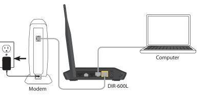
Plug the power adapter into your router and connect to an available power outlet or surge protector.
