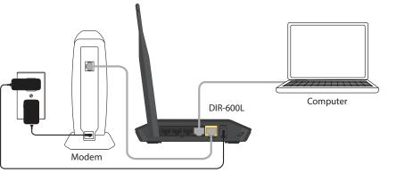
After the router has powered up, verify that the Power and Internet LEDs are both lit then continue with the *Configuration* section on the other side.
