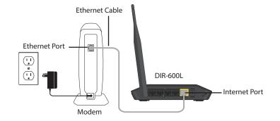
Connect another Ethernet cable from the Ethernet port on your computer Connect another Ethernet capie from to one of the LAN ports on the router.
