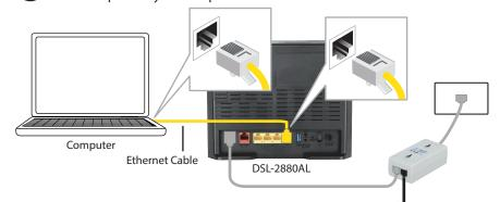
Plug the power adapter into your modem router and connect to an available power outlet.
