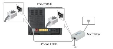
Connect the Ethernet cable from Ethernet port on your computer. Connect the Ethernet cable from the LAN port of the modem router to the
