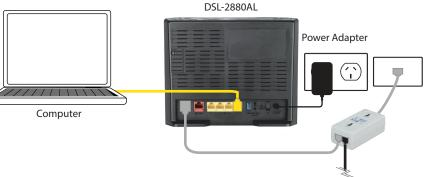
After the modem router has powered up, verify that the Power and ADSL LEDs are both lit.
