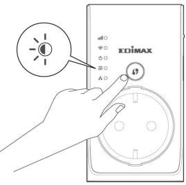
**3.** The devices will establish a connection. The extender's **green** WPS LED should display on for 5 minutes to indicate a successful connection.
