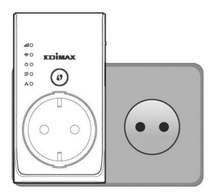
2. The green power LED will flash while the extender is starting up. The device is ready when the green power LED displays on.
