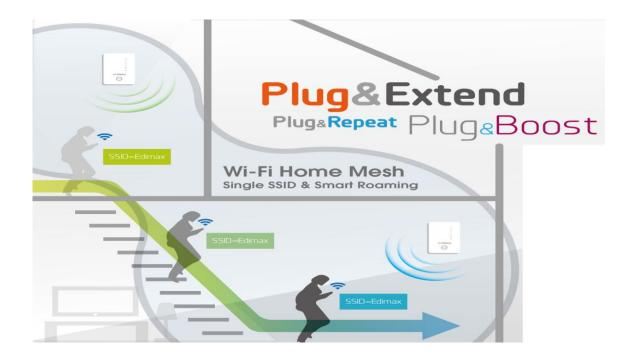
You only need to setup one extender to join your existing Wi-Fi network. This acts a master extender.
