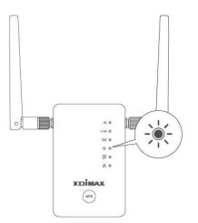
**3.** Use a Wi-Fi device to connect to the SSID "EdimaxEXT.Setup \*\*". The default Wi-Fi SSID and password is printed on the Access Key Card.
