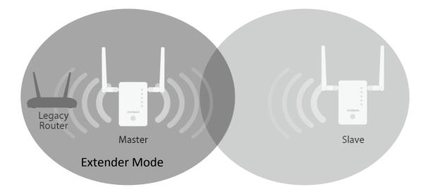
Each RE11S can function in one of three modes. To use roaming, setup your **master** extender in **Wi-Fi Extender** or **Wi-Fi Access Point** mode.
