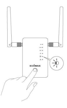
**4.** Both extenders' **green** WPS LED should display on for 30 seconds to indicate a successful connection. (If not, please restart each device and try again). Roaming will be available automatically.
