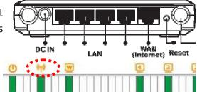
Wireless LED will be fully on when system is powered up and ready.
