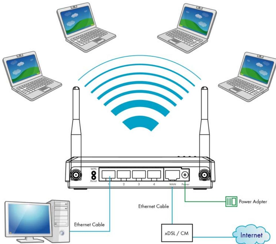
The wireless network diagram of WLAN Broadband Router..
