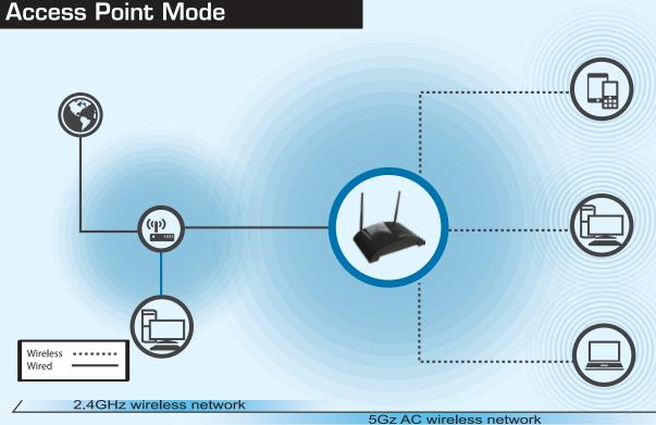
**Access Point** Mode: The HW7ACB acts as a standard wireless access point. It can upgrade your existing 2.4GHz WiFi network to a 5GHz AC or expand it, giving it greater coverage. After setup, be sure to hook the HW7ACB to your network via LAN ports 1-4.
