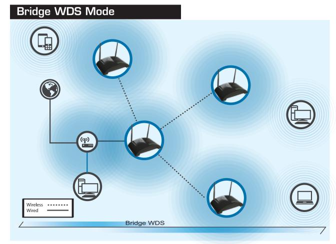
Bridge WDS Mode: The HW7ACB allows you to connect up to 4 HW7ACB's wirelessly to each other to expand the scope of your network. In this mode, the HW7ACB will transmit a wireless signal. Be sure to use the same SSID, channel and security for each. The first HW7ACB must be connected to the primary network via LAN port 1-4 and the others can be standalone.
