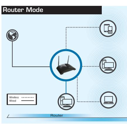
Router Mode: The HW7ACB acts as a standard wireless router and supports 2.4GHz and 5GHz AC. Use this mode to share an internet connection. Plug your modem provided by your Internet Service Provider into the port labeled WAN. Wired computers can go into LAN ports 1-4.
