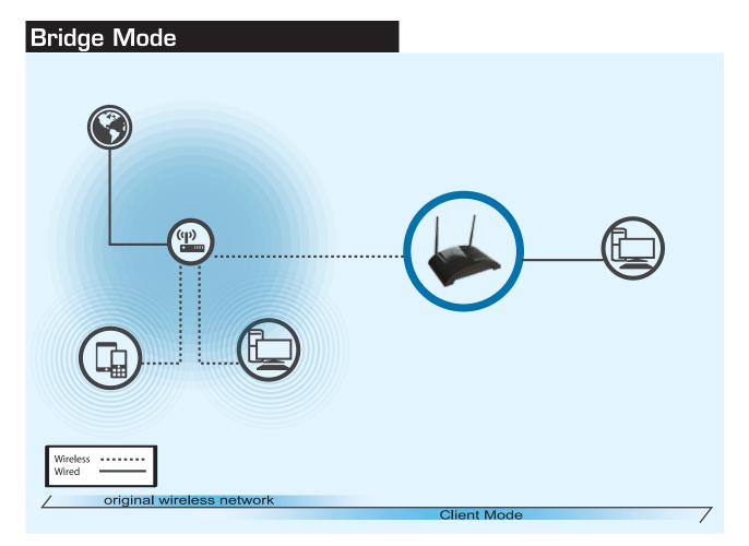
Bridge Mode: The HW7ACB allows you to connect wired devices wirelessly to an existing wireless router or access point. Non-wireless devices can network wirelessly with your Wireless Network. In this mode, the HW7ACB does not broadcast any wireless signal. After setup, be sure to hook it up to client computers/devices via LAN ports 1-4.
