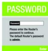
**K** Screen 8 asks you to change the password to make your Router more secure. Enter a new password, which can be between 1 and 32 characters, in the **Password** field, then repeat it in the **Confirm** field.
