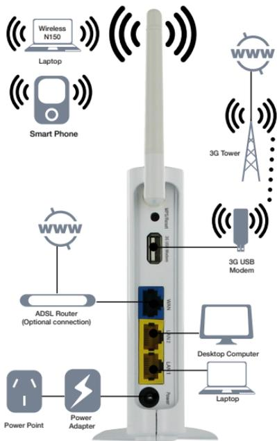
You can connect multiple wireless devices, including laptops, desktops and PDA's to your 3G17Wn by following these two basic steps.
