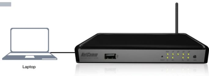
1. Connect the **yellow Ethernet cable** provided to one of the ports labelled **“LAN1-LAN4”** on the back of the NetComm 3G18WW.
