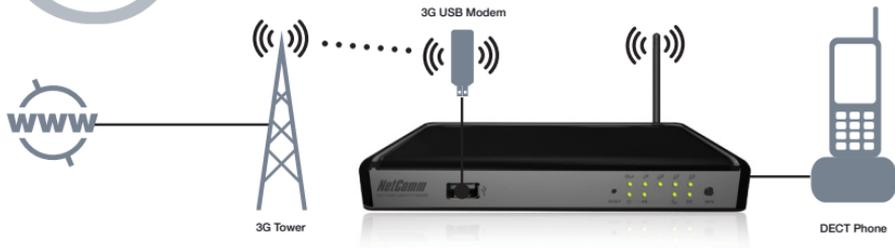
The NetComm 3G18WW allows you to make VoIP calls over the Internet by simply plugging a standard analogue telephone into the router and using a VoIP Service Provider (VSP).
