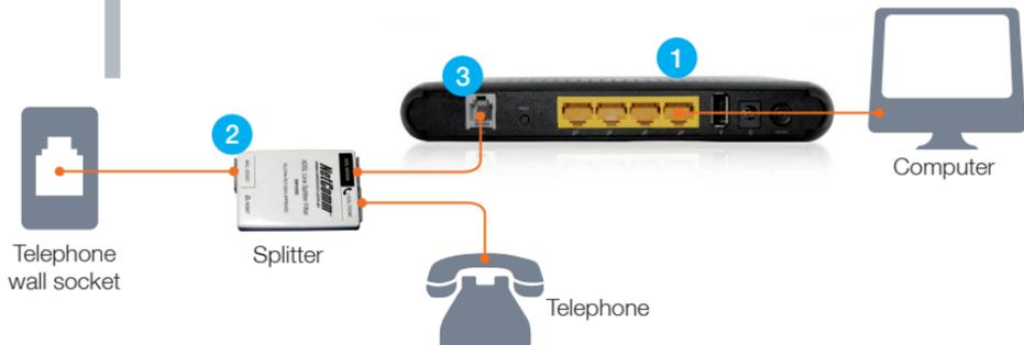
1. With the supplied Ethernet cable, connect your computer to any of the 4 LAN ports on the back of the NB304
