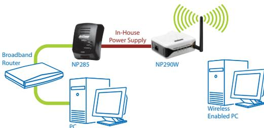
1. Insert one end of an Ethernet cable from the router's Ethernet port, then insert the other end into the HomePlug's Ethernet port .
