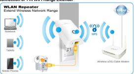
Step 1. Connect the Ethernet cable to LAN Port
