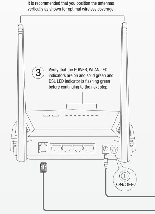
Plug the included power adapter into an available outlet and into your modem router. Then push the On/Off power button to turn on your modem router.
